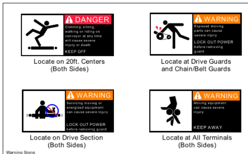
Figure 12: Safety Labels on Conveyor
