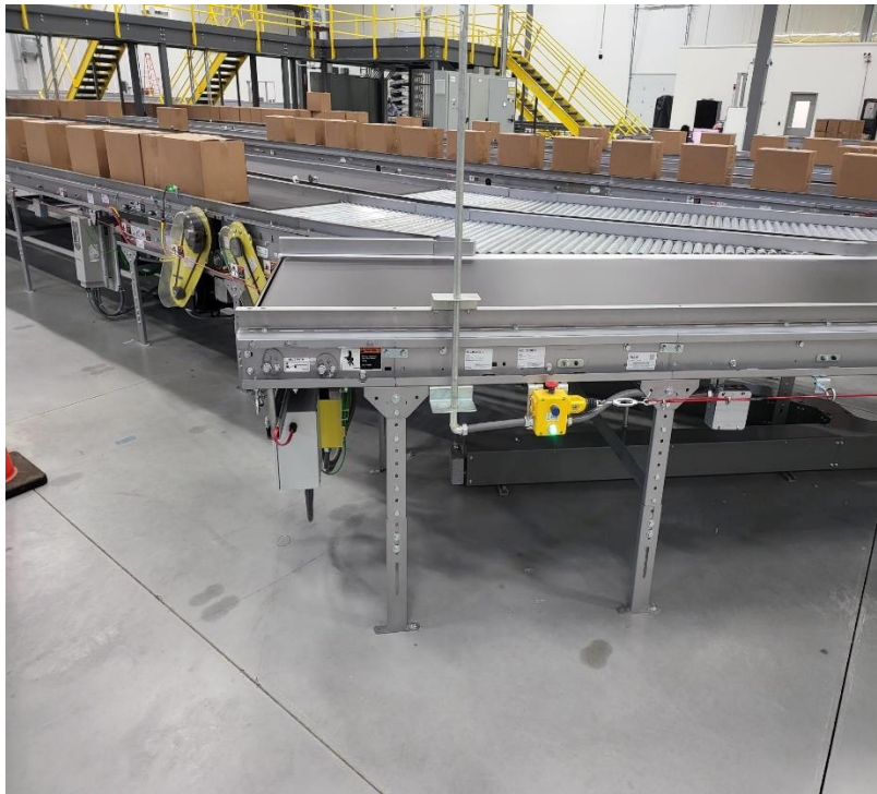
Figure 21: Support of Terminal End without Adjacent Conveyor
