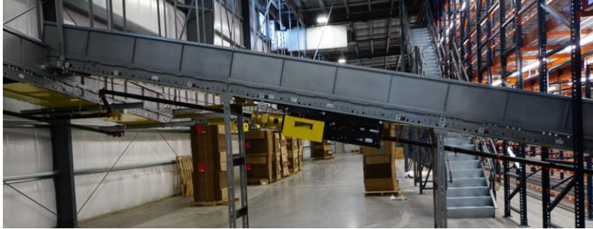
Figure 5: Empty Carton Conveyor perpendicular transition
