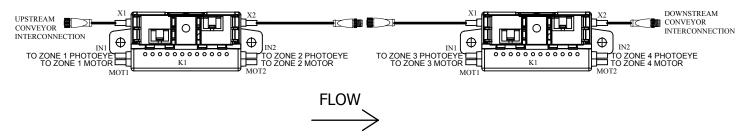
There are two types of accumulation release: Singulation release and Slug release. Singulation release allows one product to be released at a time after the downstream zone has cleared. Slug release allows a predetermined amount of product to be released at one time after the downstream zone has cleared. Slug release is typically used in Palletizing or Machine loading conditions. The type of release to be used is usually determined at design time.
