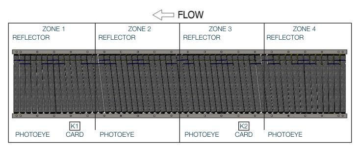
There are two types of accumulation functionality modes: Singulation release and Slug release. Singulation release allows one product to be released at a given time after the downstream zone has cleared. Slug release allows a predetermined amount of product to be released at one time after the downstream zone has cleared. Slug release is typically used in Palletizing or Machine loading conditions. The desired mode of accumulation is established by the operational needs of the conveying system.
