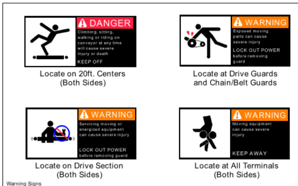
Figure 50: Safety Labels on Conveyor
