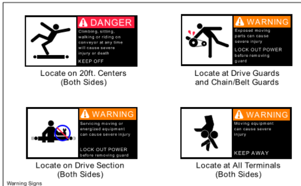
Figure 23: Safety Labels on Conveyor
