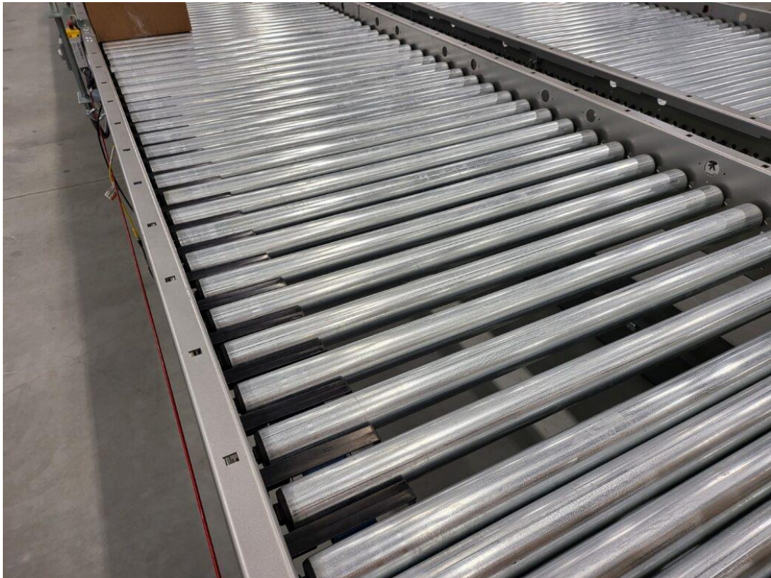
Figure 1: Narrow Belt Conveyor
