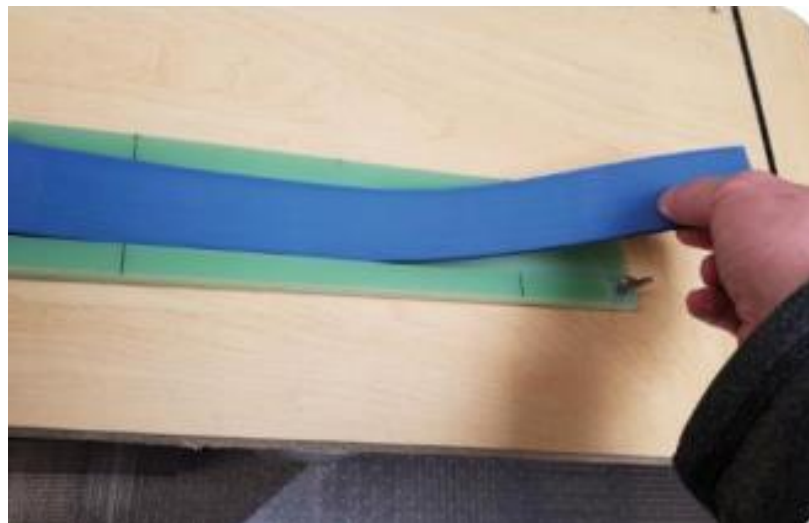
Figure 41: Remove Belt from Mold
