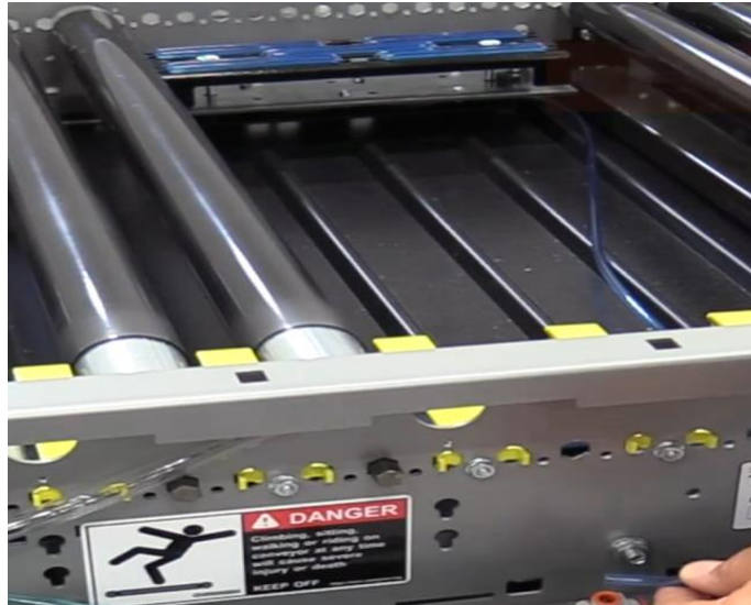
Figure 19: Installed Brake Kit
