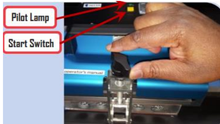
Figure 40: Pilot Lamp and Start Switch
