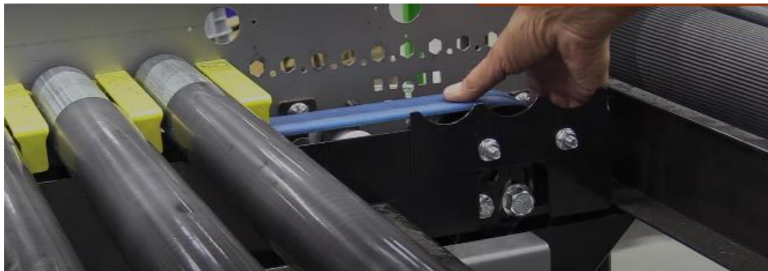
Figure 43: Checking Belt Tensioning
