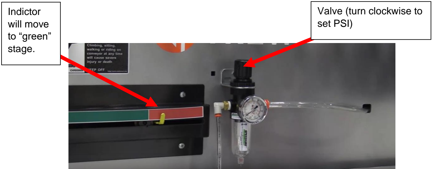
Figure 42: Air Take Up Regulator
