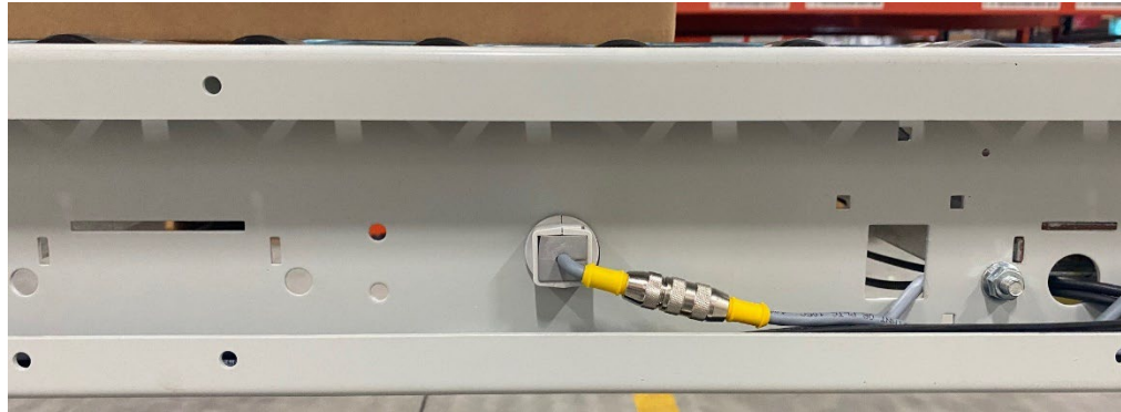
Figure 12: Wire Containment Cord Grip
