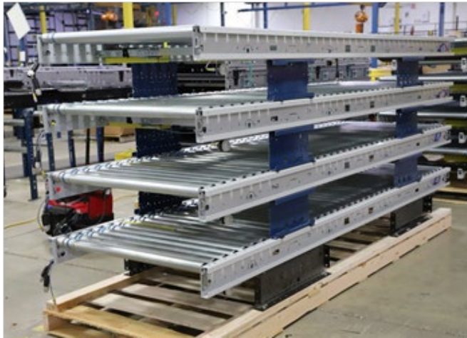
Figure 2: Stacked Conveyor Beds
