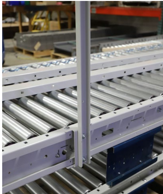
Figure 35: Cable Mast Mounting
