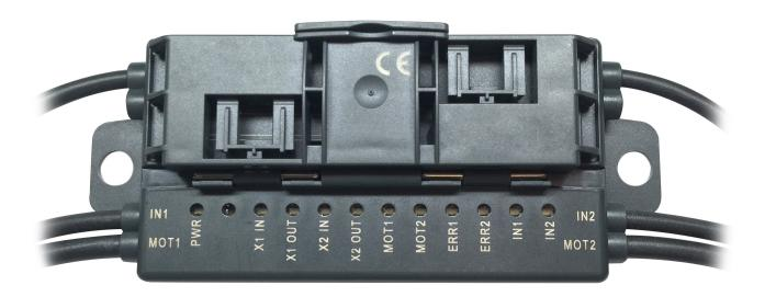
The Motor Control Module is a field module with two sensor inputs and two electronic outputs for controlling DC roller motoros. The module is optimized for use with the Interroll EC310 Motorized Drive Roller.
