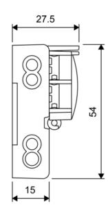
Note: The device is intended to be always mounted with its top upside, as the conveying direction is important for the wiring of the device. If the device is mounted upside down, the logical and physical conveying direction do not match, which would lead to unexpected behavior.
