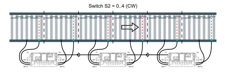
If the conveying direction is reversed, only the direction setting on switch S2 has to be changed, the cabling remains the same. The direction setting defines, which of X1 and X2 the downstream and upstream connector is.
